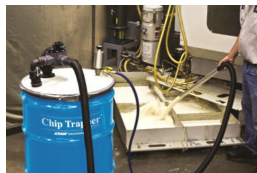
Emulsione filtrata da High Lift Chip Trapper
