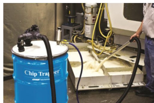
Emulsione filtrata da High Lift Chip Trapper
