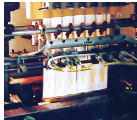
A Model 1212 12" (305mm) Standard Air Knife opens mustard packets prior to fill.
