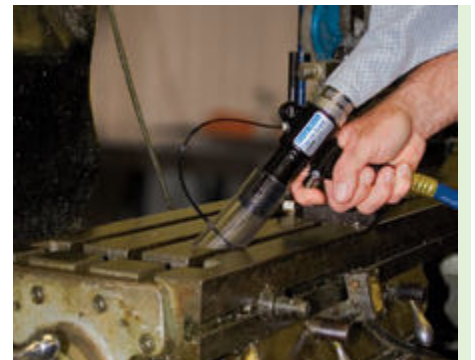
The Model 6194 Deep Hole Vac-u-Gun cleans the t-slots on a milling machine.
