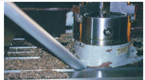
The Chip Vac removes abrasive stainless steel chips from a CNC.
