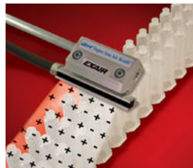
A small Model 112203 3" (76mm) Gen4 Super Ion Air Knife System eliminates contaminants from syringes prior to packaging.
