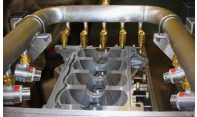
Adjustable Air Amplifiers and High Velocity Air Jets dry an engine block prior to assembly.
