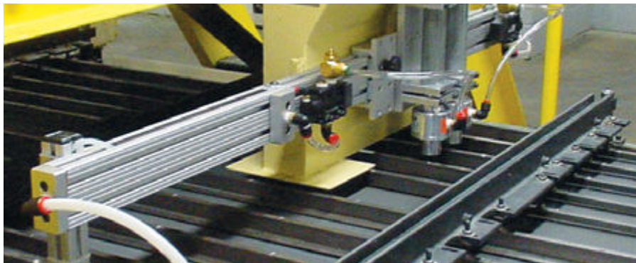
(2) Model 6083 1-1/2" (38mm) Line Vacs convey rejected metal caps from a fluorescent lamp operation to a scrap bin.
