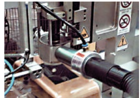
1-1/4" (32mm) Line Vac is mounted on a burr removal tool to suction the plastic shavings and transport them to a waste container.
