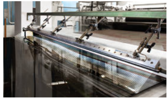
This 96" Long Gen4 Super Ion Air Knife cleans an acrylic sheet before protective wrap is applied.
