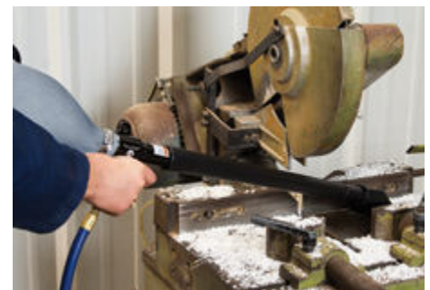
Model 6392 Vac-u-Gun All Purpose System removes plastic shavings from a saw.
