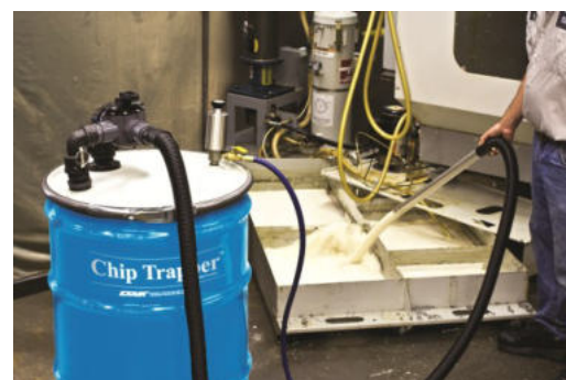
Emulsione filtrata da High Lift Chip Trapper
