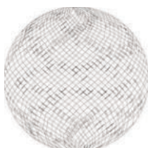
Orbitor 4 nozzle spray pattern
