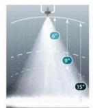
1/8 NPT Siphon Fed Flat Fan atomizing nozzles apply a light coating of liquid over a wide band.
