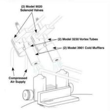
The Problem: Air conditioner parts assembled on an automatic brazing machine must be cooled to handling temperature prior to removal. The machine was capable of brazing up to four hundred pieces per hour. However, the time required for the parts to cool severely limited the production rate. Water cooling was unacceptable from the standpoint of both housekeeping and part contamination.
