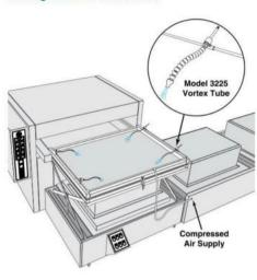
The Problem: A manufacturer of major appliances vacuum forms the plastic interior shell of refrigerators. The deep draw of the plastic and complex geometry left the four corners unacceptably thin. The corners would tear during assembly or bulge when insulation was inserted between the shell and exterior housing, resulting in a high rejection rate.
