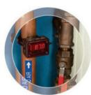
Pressure Sensing Digital Flowmeters monitor pressure and flow. A pressure sensor is mounted between the two flow sensing probes. The pressure signal is provided as a second milliamp output. The display can be configured to show pressure or flow. The pressure signal is also available through wired or wireless serial outputs. The pulse output is replaced with a transistor output configured as a low-pressure alarm when the pressure drops below 50 PSIG. Available on 2" and 50mm or larger flowmeters.
