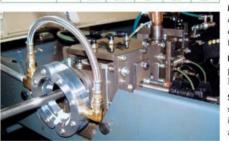
The Super Air Wipe eliminates the possibility of smoke during machining by wiping hydraulic oil from the bar stock as it enters
