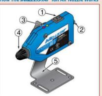
After connecting the 24V power supply, activate the power switch (1) and turn on a compressed air source to supply the 6mm push-in fitting (2) to activate the static eliminating ions and airflow. Proper or improper functionality is indicated by a green or red LED (3). The non-marring nozzle (4) provides quiet performance and OSHA compliance. The compact mounting bracket (5) is included to provide handsfree operation.
