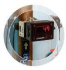
Hot Tap This meter allows for installation under pressure, eliminating the need to isolate and remove pressure from the pipe it is being installed upon. It incorporates two valves that the probes pass through and a muffler that collects chips from the drilling process. It takes an equally short amount of installation time as the standard meters. Available on 2" and 50mm or larger flowmeters.
