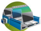
The timer was set to the "interval" setting when detecting the flat panel displays. The sensor was mounted 1" (25mm) prior to the Super Ion Air Knife blowoff station. When it detected the flat panel, it turned the air on immediately and started the 10 second timing sequence for closing the valve (shutting the air off). In the event the conveyor stopped, the air would no longer cycle on again until the next flat panel was detected.
