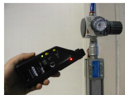
Kit Ultrasonic Leak Detector
