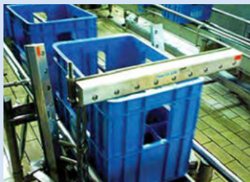
Three Model 110018 18" (457mm) Super Air Knives completely surround and blowoff crates so they can be loaded immediately.
