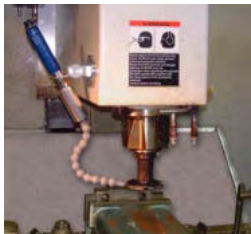
The Adjustable Spot Cooler replaces fluid coolant and eliminates hours of cleanup on a cast iron machining operation.
