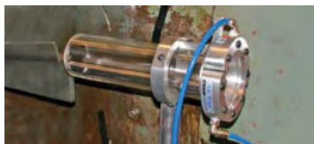
The Standard Air Wipe blows coolant off the part and back into the centerless grinder.
