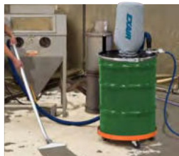
Sand that covers the floor around a sand blaster is quickly vacuumed into the drum using the rugged floor tool.
