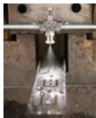
Model EF8010SS applies lubricant to a drawer slide.
