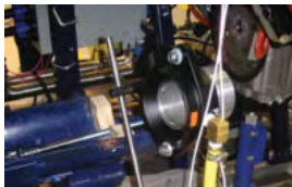
A Model 120024 4" (102mm) Super Air Amplifier cools an engine during dynamometer testing.
