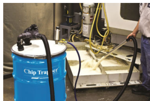
Emulsione filtrata da High Lift Chip Trapper
