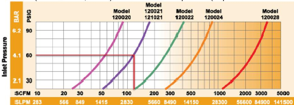
Total Output Flow with .003" (.08mm) thick shim installed. Excludes downstream entrainment.
