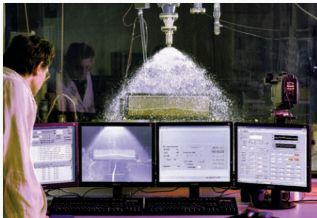
The BETE Droplet Analyzer is capable of characterizing non-spherical droplets like those seen in this actual image.
