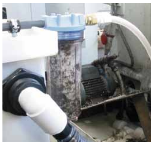
Filtro primario rimozione particelle solide Primary filter traps chips and solid bodies
